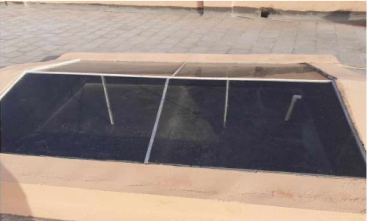
Fig 14: Distilled water solar still
